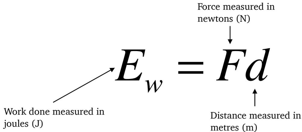
The diagram shows the formula  $E_w = Fd$  in a large, bold, serif font. An arrow points from the text 'Work done measured in joules (J)' to the  $E_w$  term. Another arrow points from the text 'Force measured in newtons (N)' down to the  $F$  term. A third arrow points from the text 'Distance measured in metres (m)' up to the  $d$  term.
